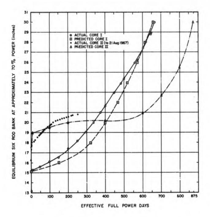
Figure 2. Core Life versus Six-Rod Bank, PM-1, Cores I and II
