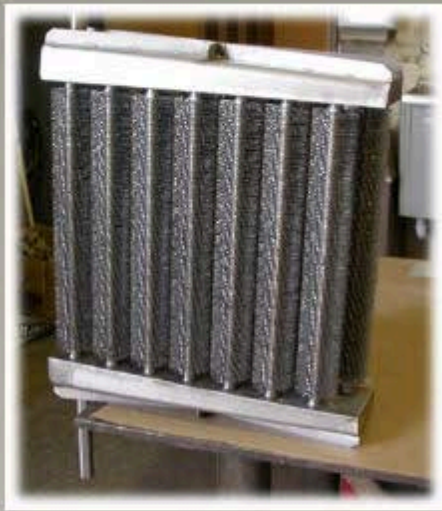
Finned tube air cooler - 200 kw
