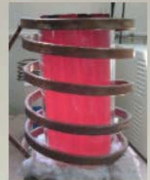
Inductive heating of test section - 200 kw
